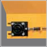
Spring loaded front idler adjustments
