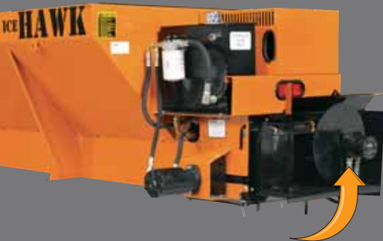
Swing up spinner assembly simplifies clean up and storage
