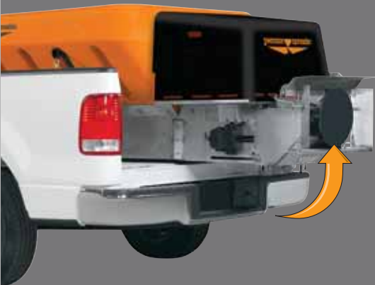
Swing up spinner assembly simplifies clean up and storage
