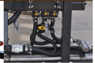
Electronic ball valves close quickly and completely eliminating excessive nozzle dripping.
