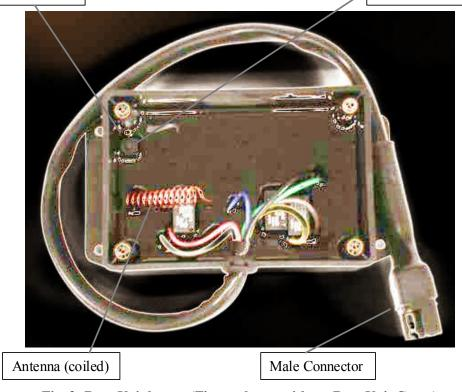
Fig. 3: Base Unit layout (Figure shown without Base Unit Cover)
