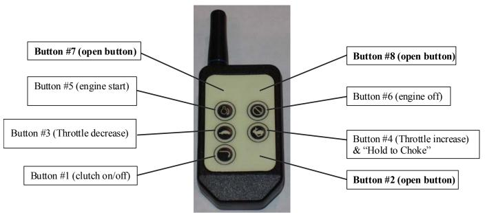
Fig. 1: Transmitter Front Button Assignments
